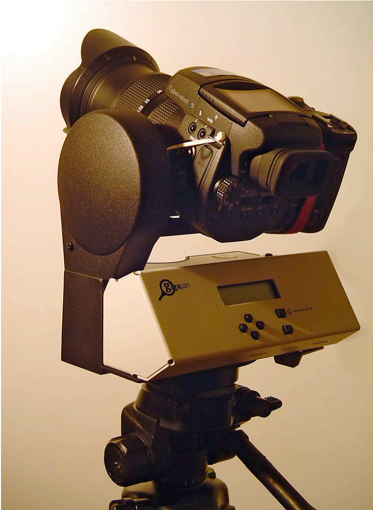
Figure 2-75. A Gigapan imager mounted with a Sony DSC R1. (Courtesy Wikimedia Commons, under the GNU Free Documentation License.)
